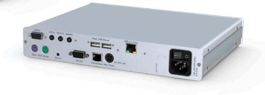
links: CATVision-ARU2D-CPU Rechnermodul
