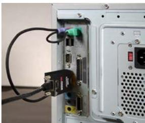
Direct connect CAT5 Transmitter streamlines your installation
